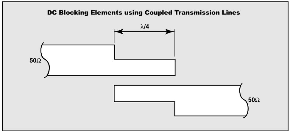
Figure 9. Coupled Microstrip Transmission Line DC Block
