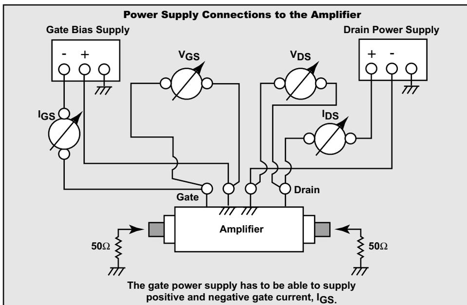
**Figure 1. Power Supply Connections to the Amplifier**
