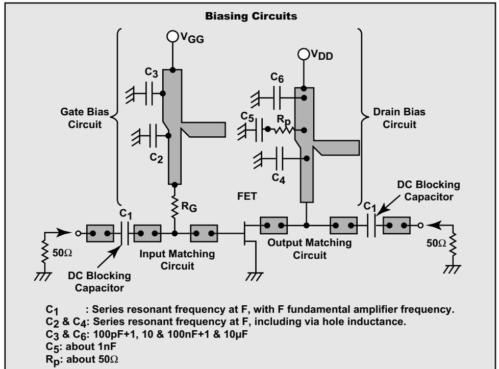
Figure 4. Amplifier Block Diagram
