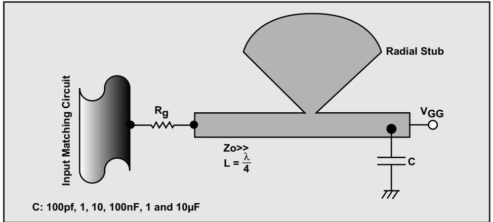
Figure 8. Input Bias Circuit using a Radial Stub
