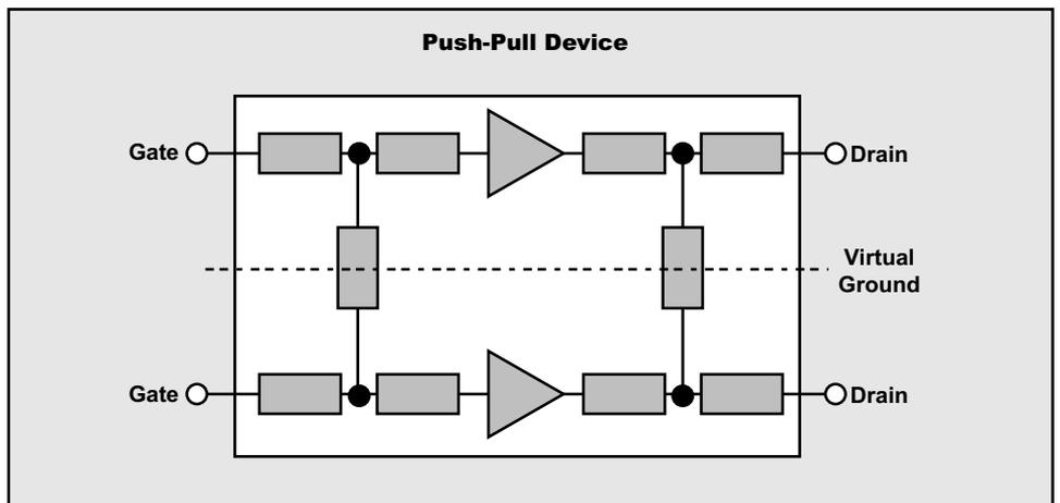
Figure 11. Real Push-Pull Device
