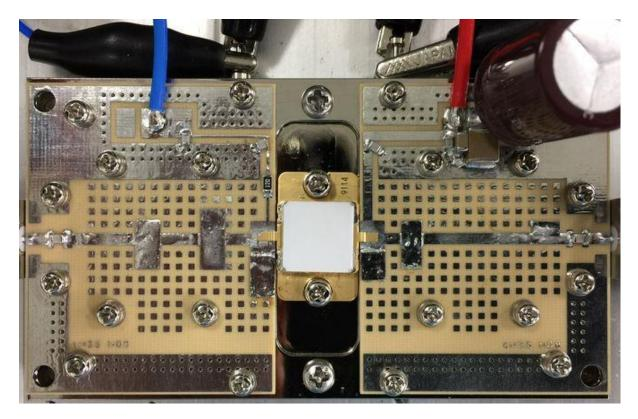
PCB: h=0.8mm, er=3.5, Cu=18µm
