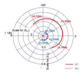
Bias Condition  $V_{DS}$ =24V,  $I_{DS(DC)}$ =1.2A Rg = 100ohm
